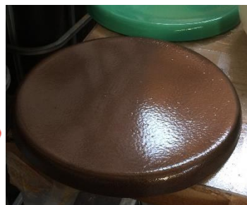
Apply Conventional Car Paint. Substrate colour will be invisible. (This time we used “Brown-Gold Base car Paint ”)
